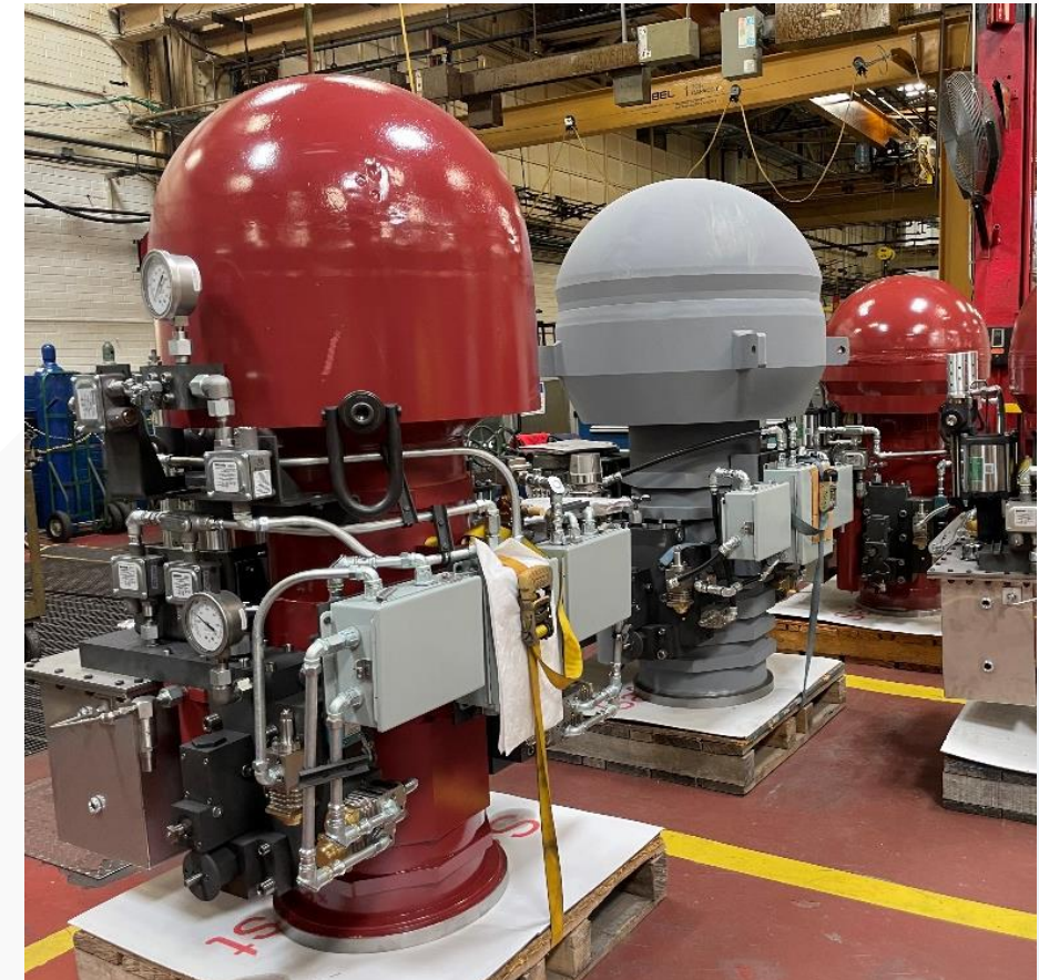
Nuclear actuation for Main Steam Isolation Valves (MSIV)
