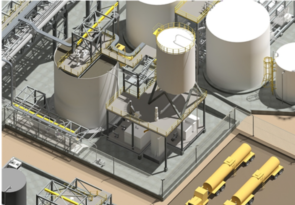
Figure 24-13: Lime Slaking System
