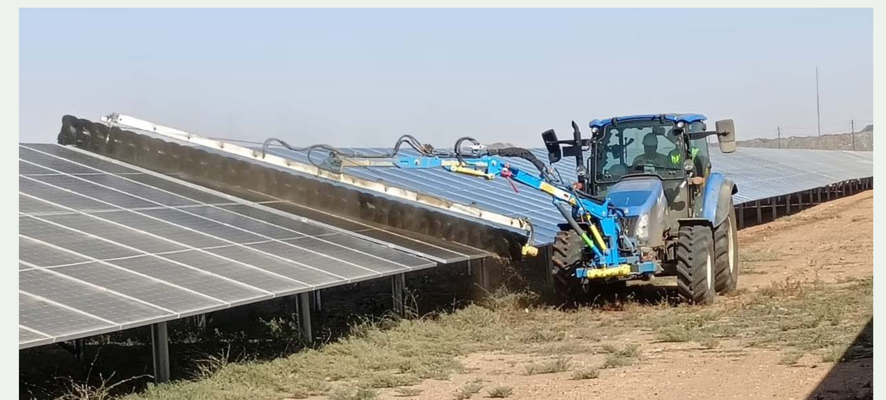
At Tasiast, we have invested in a mechanical cleaning system to manage dust levels efficiently.
