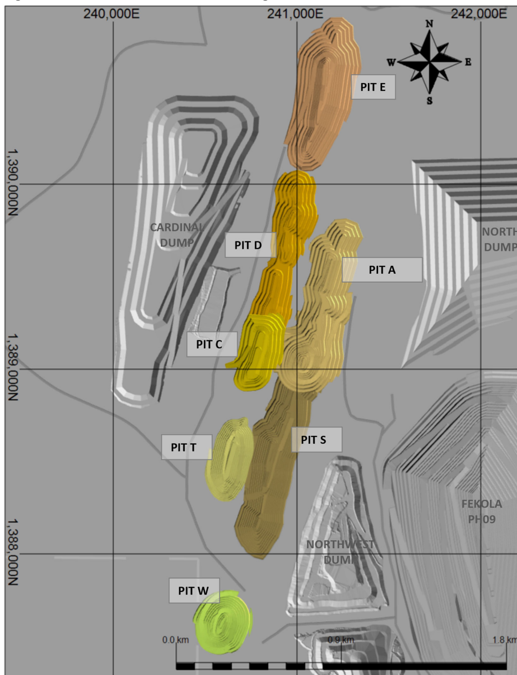
Figure 15-2: Cardinal Zone Pit Phase Design
