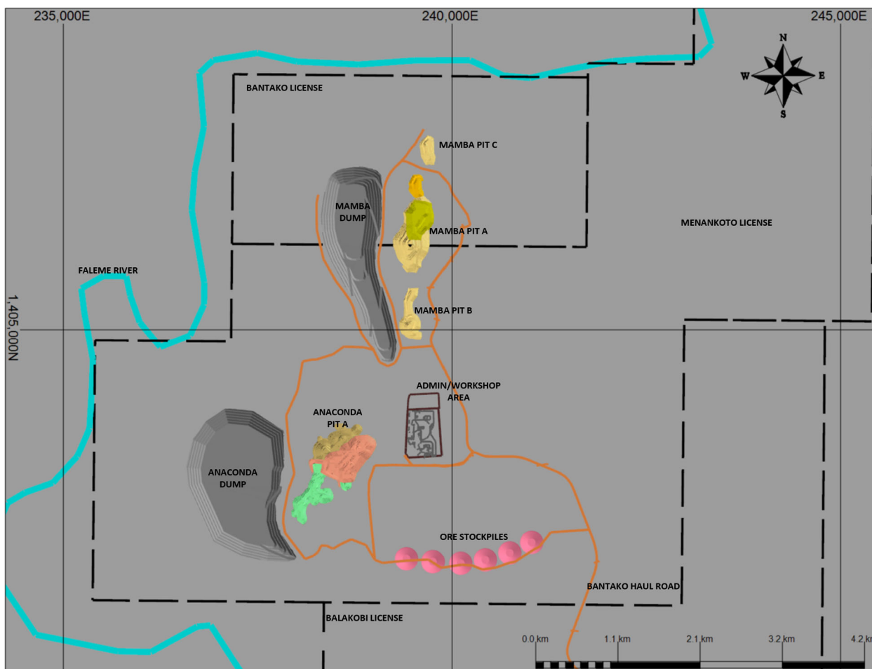
Figure 18-3: Infrastructure Layout Plan, Anaconda Area
