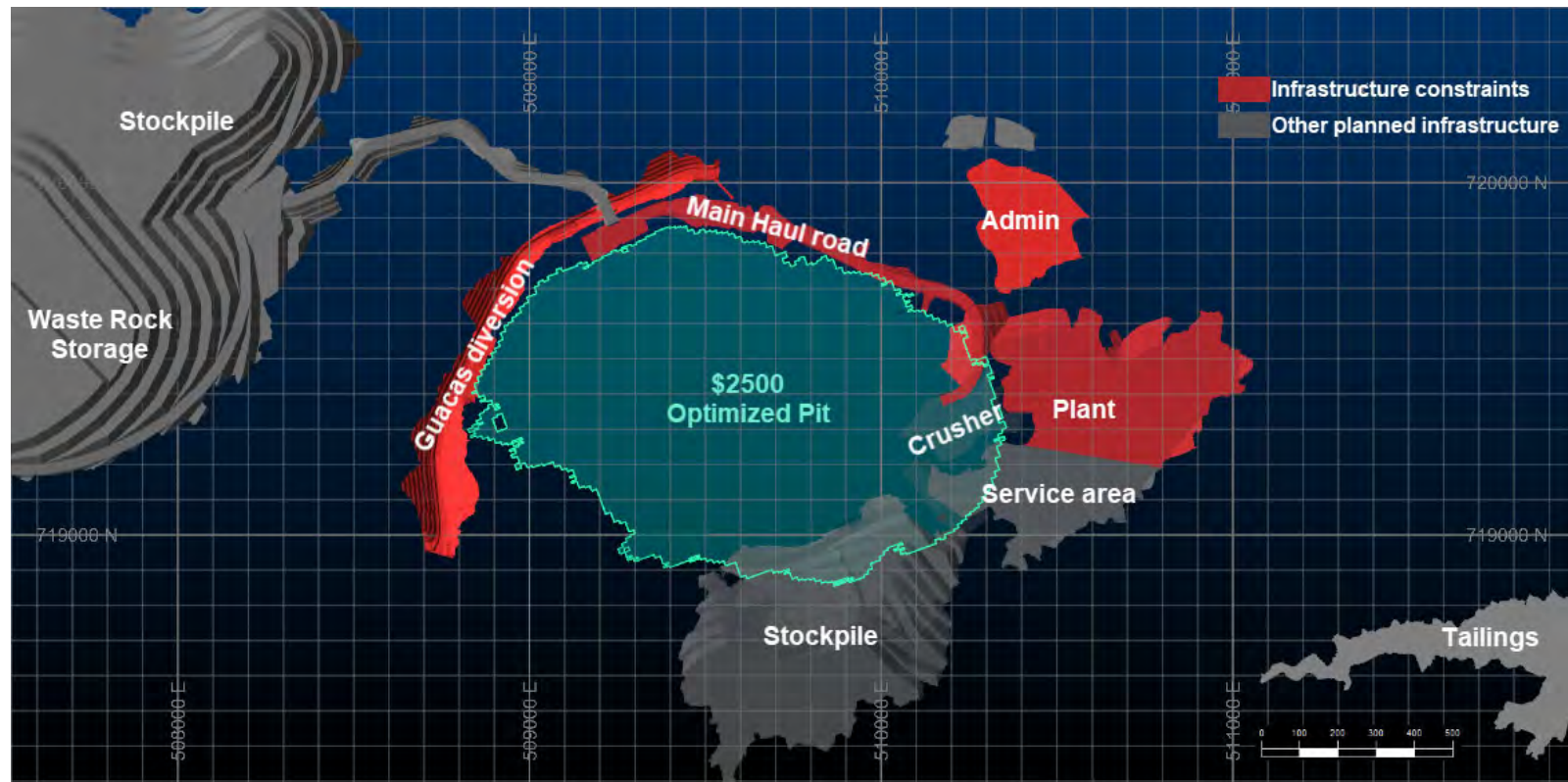
Figure 14-4: Infrastructure Constraints To Pit Optimization
